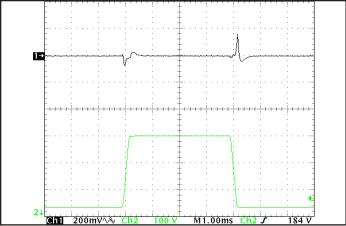
Figure 12: Output voltage response to step-change in input voltage (250V/ms). Load cap: 100 μF electrolytic output capacitance. Ch 1: Vout (200mV/div), Ch 2: Vin (100V/div). Timescale: 1.00ms/div.
