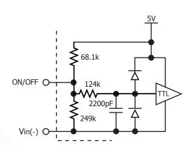
Figure B: Internal ON/OFF pin circuitry
