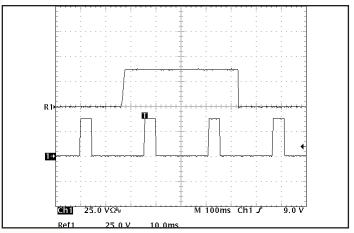
Figure 18: Load current (25A/div) as a function of time (10ms/div and 100ms/div) when the converter attempts to turn on into a  $10m\Omega$  short circuit.
