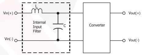
Figure E: Internal Input Filter Diagram
