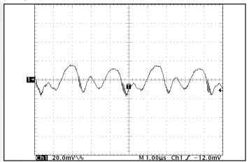
**Figure 10:** Output voltage ripple, Vout, at nominal input voltage and rated load current (20 mV/div). Load capacitance: 1µF ceramic capacitor and 10µF tantalum capacitor. Bandwidth: 10 MHz. Timescale: 1.00µs/div. See Figure 17.
