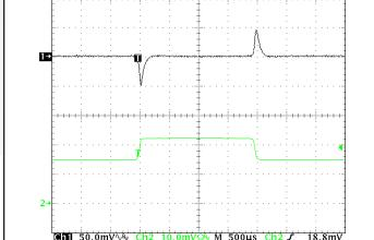
Figure 11: Output voltage response to step-change in load current (50%-75%-50% of Iout(max); dI/dt = 0.1 A/μs). Load cap: 1 μF ceramic and 15 μF tantalum capacitors. Ch 1: Vout (50mV/div), Ch 2: Iout (10A/div). Timescale: 500μs/div.
