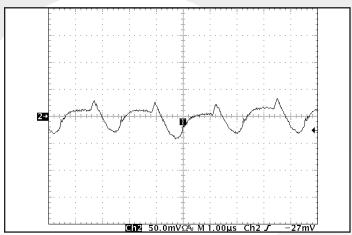
Figure 9: Input terminal current ripple, i<sub>C</sub>, at full rated output current and nominal input voltage with SynQor MCOTS filter module (50 mA/div). Bandwidth: 20MHz. Timescale: 1.00µs/div. See Figure 17.
