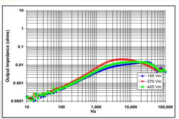
Figure 13: Magnitude of incremental output impedance ( $Z_{out} = v_{out}$ ) for minimum, nominal, and maximum input voltage at full rated power.
